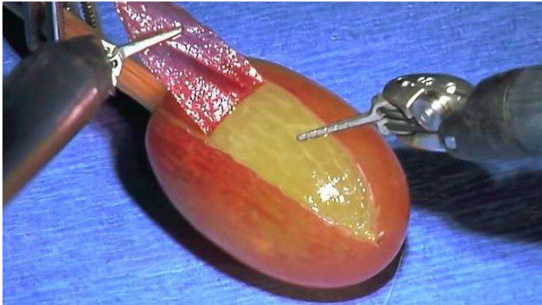
Figure 2: da Vinci Surgical System performing surgery on a grape, showcasing its steadiness and preciseness 16
